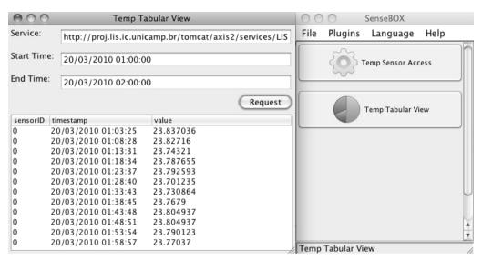
Figure 5 – Application visualizing Temperature sensor data in a data table.
